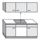
When two or more appliances are installed together below a cooker hood, e.g. a gas wok and a ceramic hob, which have different safety distances given in the installation instructions, you should select the greater distance of the two.
